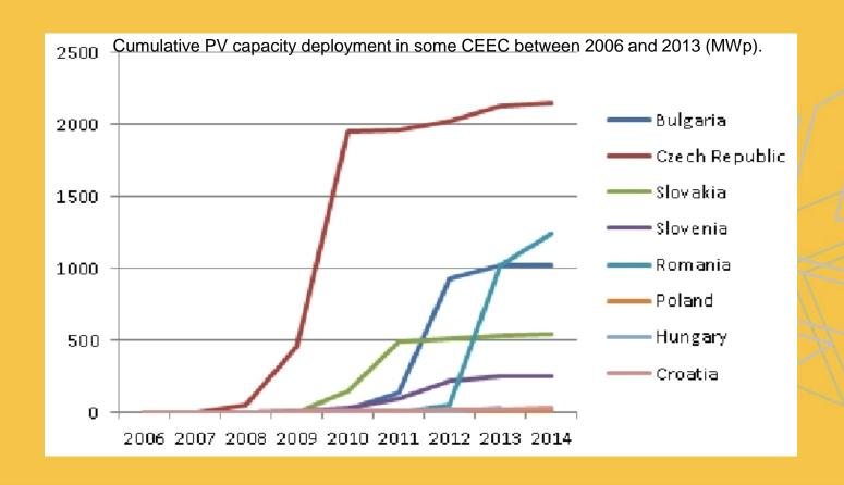
Source: Dusonchet, L.– Telaretti, E. (2010); Photovoltaic energy barometer 2007, 2009, 2010, 2011, 2012, 2013 – EurObserv'ER, and http://photon.info data own edition
